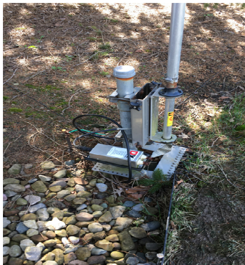
Closeup of Hustler 5-BTV Mounting and Radial System
